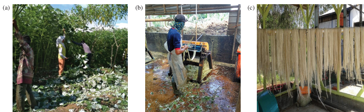
Fig. 1. Ramie fiber processing (a) ramie harvesting (b) ramie fiber decortication (c) ramie fiber naturally drying.
